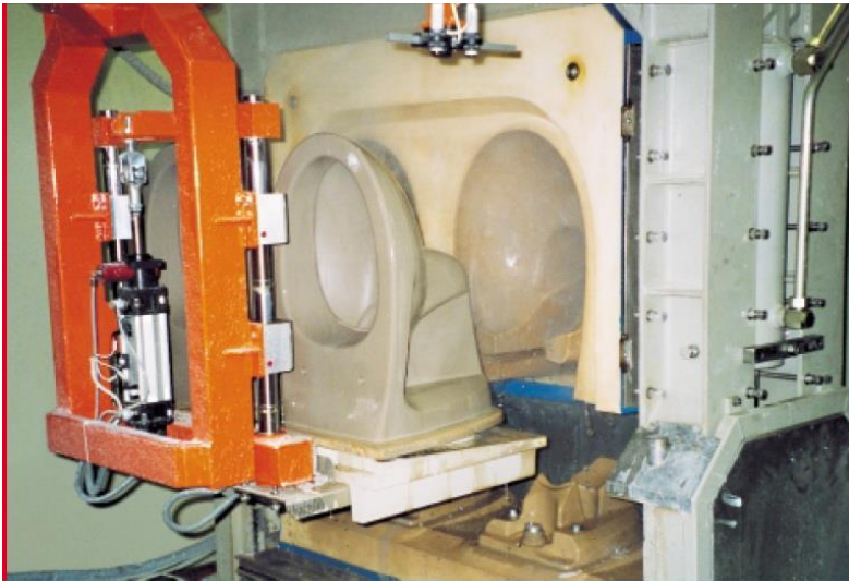
Fig. 15. Stand for high-pressure casting of sanitary ware in acrylic forms (Sacmi Forni).
